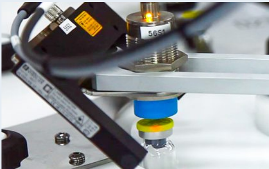
Missing alum. cap check / crooked cap check
