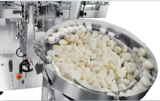
Automatic unscrambling vibrators for plastic foam
